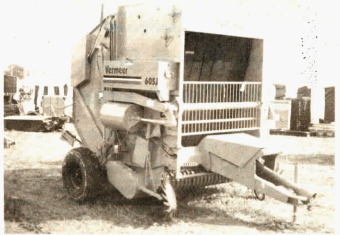
"Robot baler" features automatic steering and air-bag springs, (see side of baler in photo) that provide uniform bale density at an infinite range of pressure settings.
