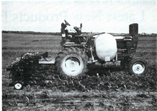
Augustine cut off the cab, moved the seat and controls to the center of the machine, and widened the wheelbase to 120 in.
