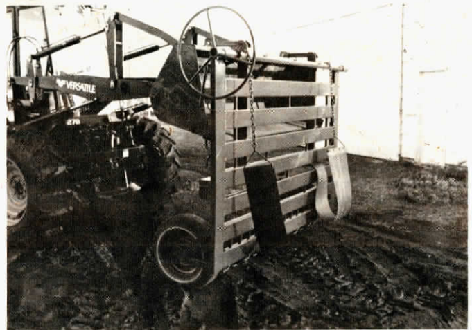
Held upright by loader, the new trimming chute rides on two 15-in. tires.
