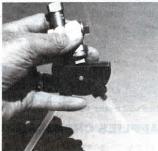
"Accu-Set" duplicates the spray pattern so you can set nozzles for height, angle and proper coverage without turning on the sprayer.
