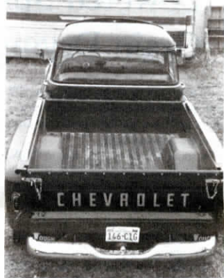
Owens fitted his home-built pickup with the floor and fender wells out of a 1974 Chevy and the tailgate from a 1966 Chevy.
