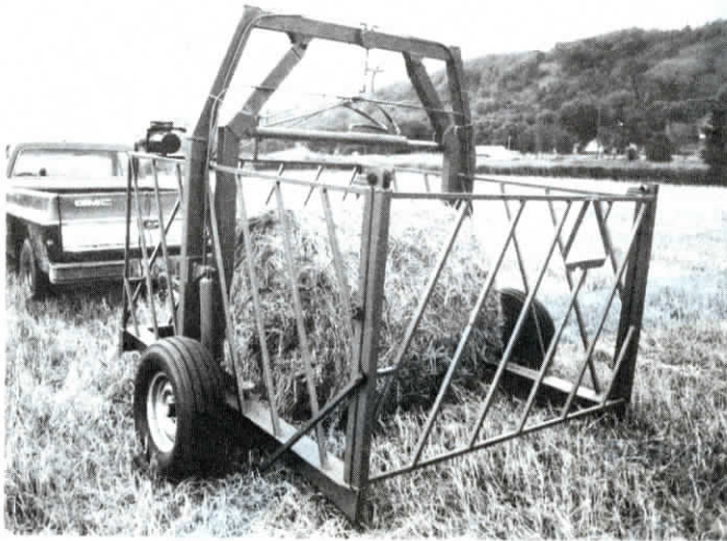
New bale hauler-feeder grabs the ends of bale with overhead "squeeze arms". It's available in 1 to 5-bale models. Feeder panels can be removed when not needed.
