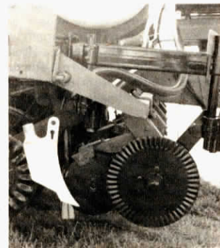
A 17-in. dia. couler mounts ahead of narrow profile knife.
