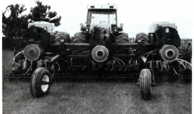
Perkins clamped 24 Yetter no-till coulters to 20-ft. toolbar fitted with three 8-row Cyclo blower units.
