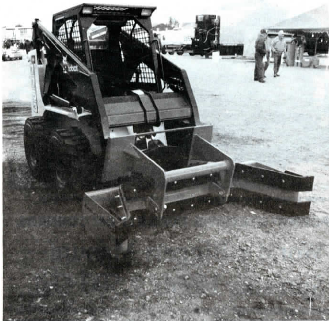
Reversible slurry blade flips over when you raise it in the air so you can operate it in the opposite direction. Note rubber strips on top and bottom of blade.
