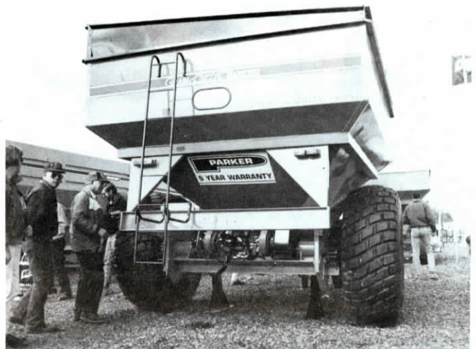
Free-wheeling, on-demand drive system can be engaged or disengaged on the go.
