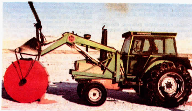
Dispenser readily adapts to front-end tractor loaders.
