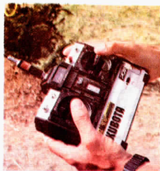
Effective range of hand-held control panel is 300 ft.
