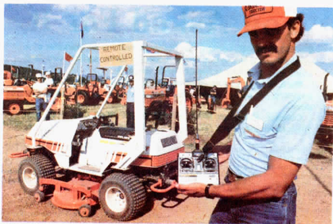
Dan Kilgas operates driverless mower using hand-held control panel.
