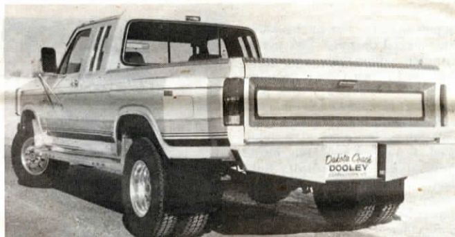
Kit consists of dual wheel spacer, outer wheel, and wide flare fender.
