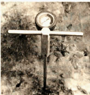
Dial on compaction tester reads out lbs./sq. in.
