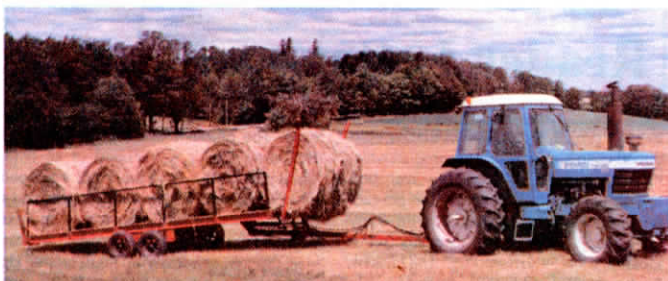
Trailer swings out to side of tractor and fork slips under bale, lifting it onto permanently tilted trailer bed.
