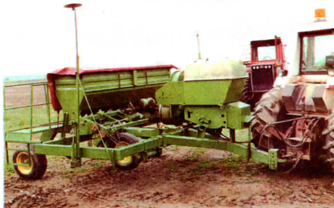
Moore fit his home-built drill with an IH Cyclo air planter system, an Oliver drill box, and the front gang of openers off a Deere 750 drill (not shown).
