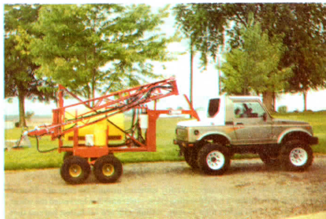
Suzuki Samurai is fitted with specially built molded fiberglass cab.
