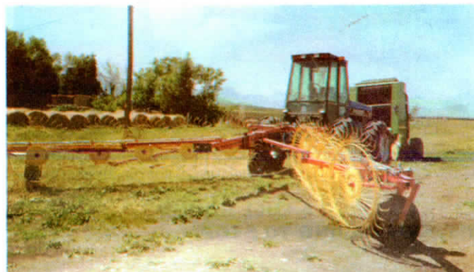
Jones mounted 10-wheel rake on "front" of his Ford Versatile 9030 Bi-Directional tractor and pulls a Deere round baler behind so he can rake and bale at same time.
