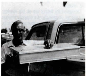
Twin toolboxes slide to the pickup sides on a common mounting rail for easy access to tools, says inventor Harold Fratzke.
