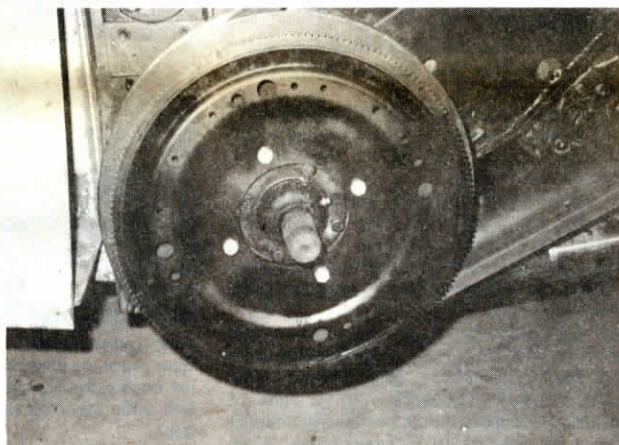
Ford flywheel bolts to variable speed drive pulley on combine.
