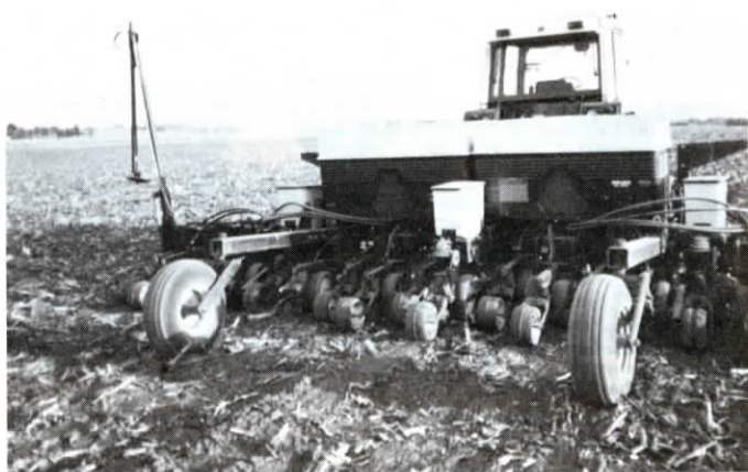
Powell says his 15-in. planter offers more accurate seed placement and better row spacing than a grain drill and does a better job handling residue.
