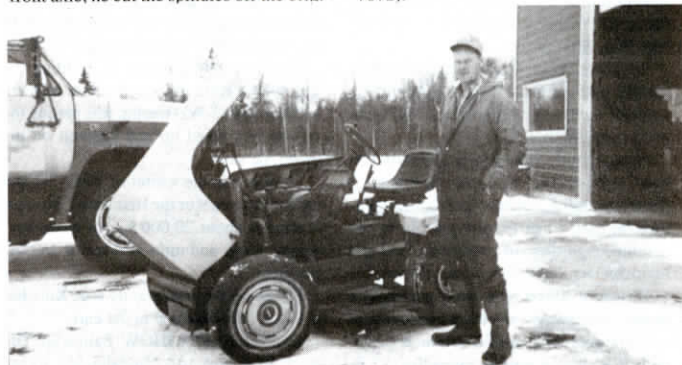
Mower is powered by a 4-cyl., 70 hp diesel engine out of a 1984 Mazda B2200 pickup.
