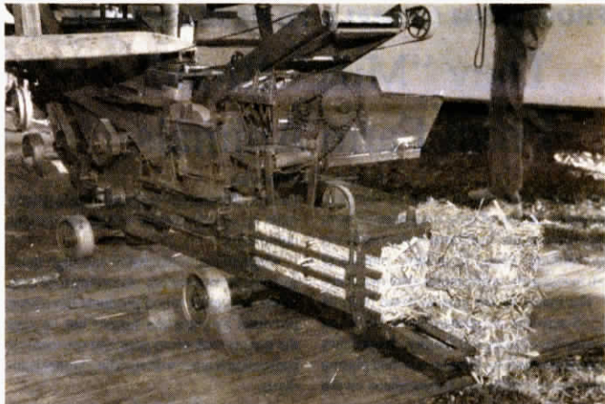
Miniature thresher feeds straw into hopper on top of mini baler that makes 6-in. bales.
