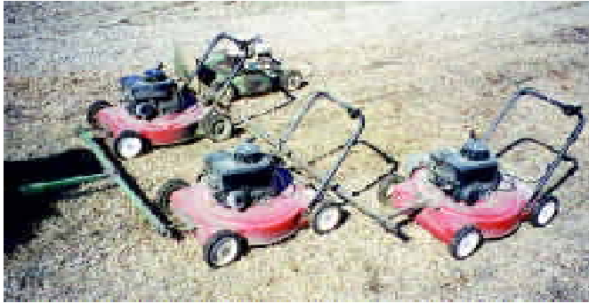
Home-built hitch allows Dyck to pull four mowers behind his riding mower. It cut his mowing time from six hours down to an hour and a half.
