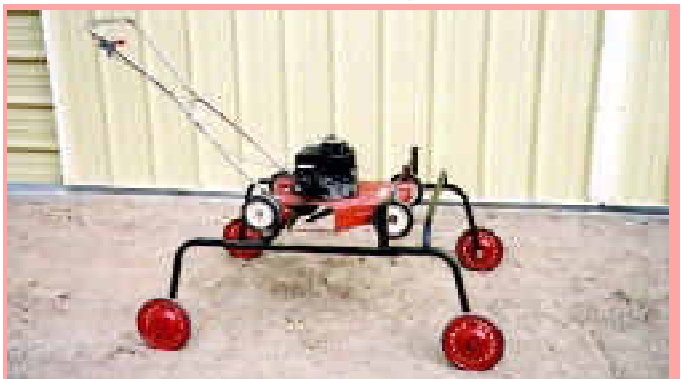
Russell mounted his 20-in. lawn mower on a height adjustable rolling carriage. To use, he positions the deck on one side of frame and pushes rig over the hedge.
