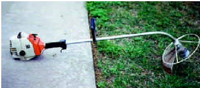
Lenart modified his Stihl "Weed Eater" by mounting a steel ring on the shaft just above the head. Ring serves as a cutting guide.
