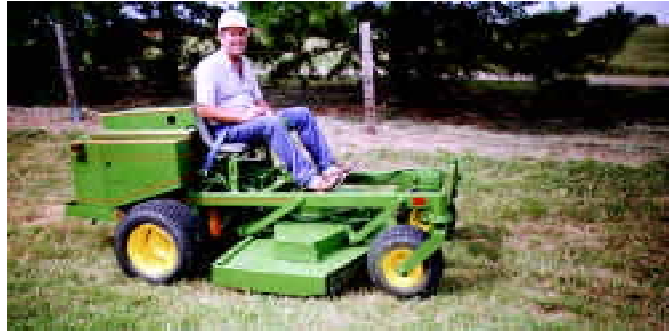
Krueger built this mower for less than $2,000. It's powered by a 4-cyl., 30 hp Continental water-cooled engine. He uses two levers in front to steer.
