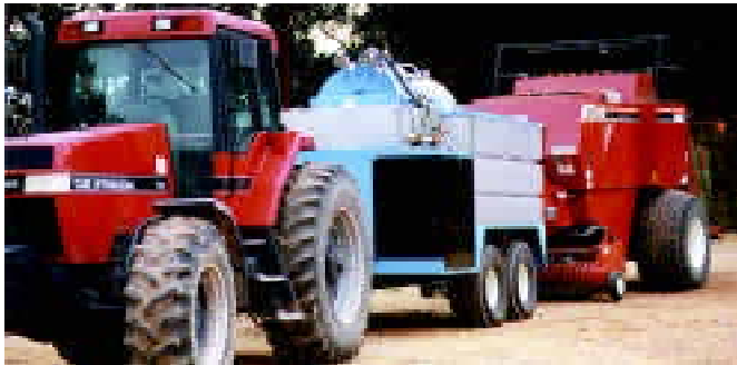
Staheli offers two models - one for use with 3-string balers and one for use with the Hesston 4900 1-ton baler. When a centerline baler is used, a video camera is mounted on back of the steam generator with a monitor inside the cab.
