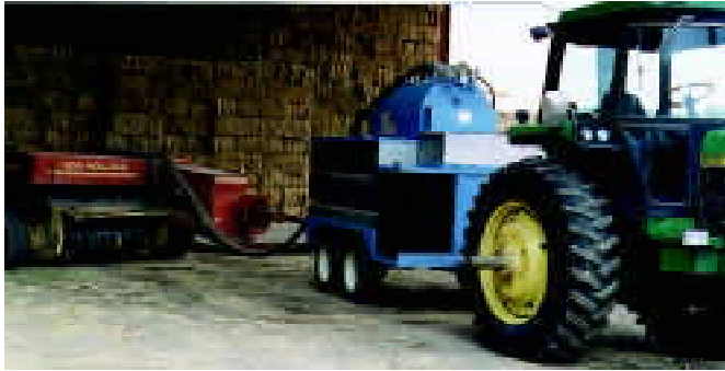
Trailer-mounted steam generator hooks up between tractor and baler. A pto shaft and hydraulic lines run through the trailer chassis back to baler.
