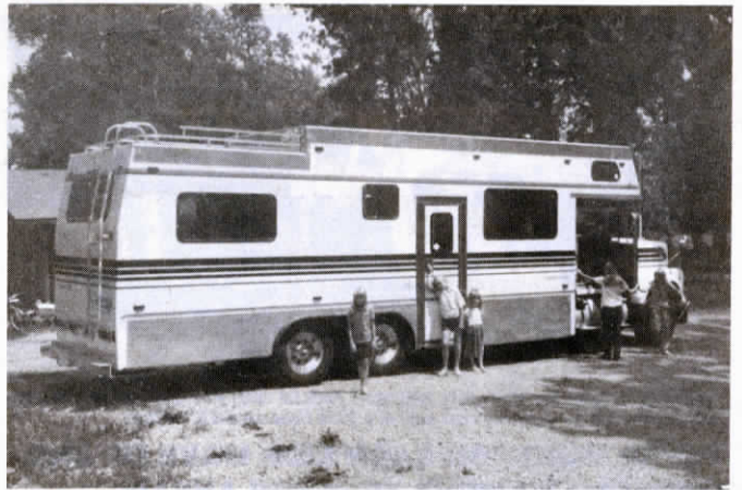
Baer used cab and tandem axle trailer frame from International 4300 semi tractor to build 37-ft. long camper. It's powered by a 400 hp Cummins 6-cyl. diesel engine.
