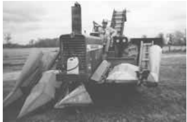
Lively mounted the 4-row corn picker on his IH 856 tractor, using the picking units off an old Allis-Chalmers combine.
