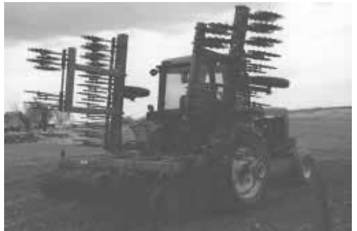
Hoe's 5-ft. wings fold up vertically for transport. A pair of depth gauge wheels controls depth of front hoe wheels. Depth of rear gangs is controlled by top link on 3-pt. hitch.
