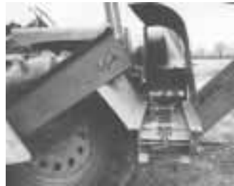
A pair of 6-ft. long home-built elevators deliver corn into cross augers (above), which deliver corn into 16-ft. long, 18-in. wide discharge elevator.
