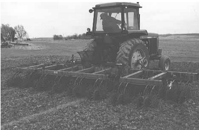
Gebhart converted a 20-ft. wide Deere rotary hoe into a "double toolbar" folding hoe that has twice as much soil mixing action as a conventional rotary hoe.
