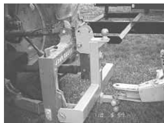
Unit has gooseneck ball hitch on top and square receiver tube at bottom that's fitted with two different sizes of ball hitches.
