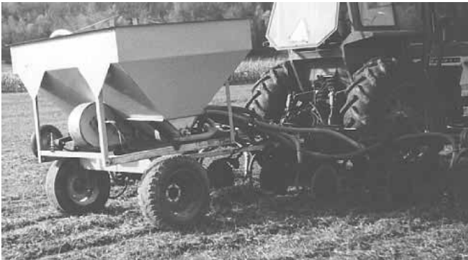
Cart can be used to do everything from deep banding fertilizer to planting soybeans.
