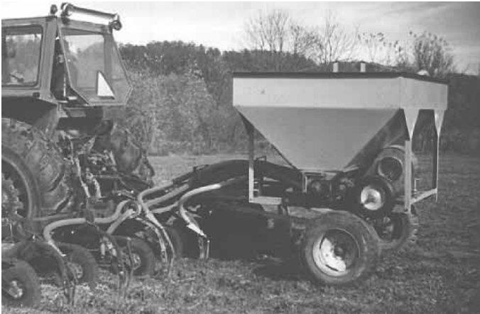
Cart is equipped with steering arm that runs from the axle to a ball hitch that mounts on toolbar pulling the cart. Keeps cart from pulling to left or right and turns precisely.
