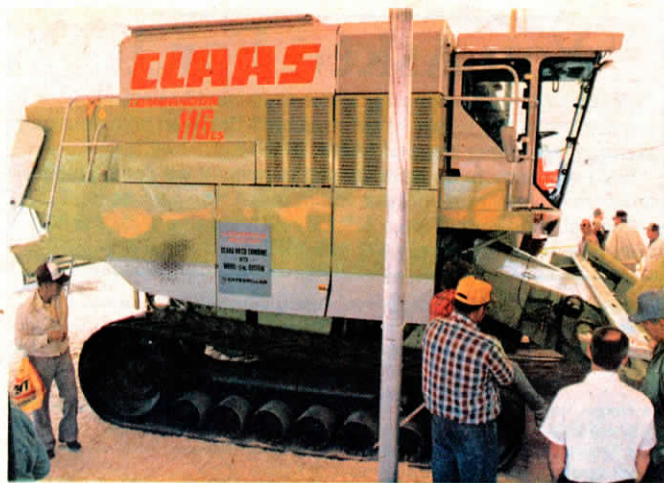
This Claas combine, fitted with new "cat tracks", showed up at the Farm Progress Show this fall in Iowa. The tracks virtually eliminate compaction, cutting ground pressure to 7 lbs. per sq. in.
