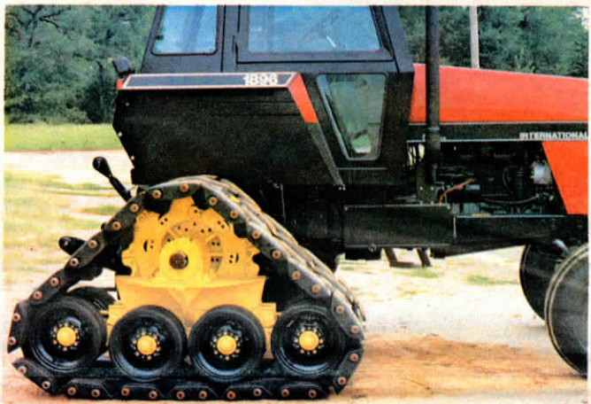
Martintrac tracks use 6-in. wide rubber cleats in place of steel grousers. The self-cleaning cleats flex like a tire to grip the ground.
