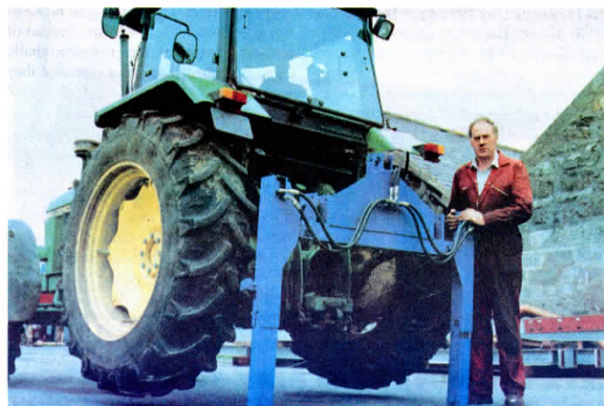
Steel legs each contain hydraulic cylinder. Pair of valves on back of frame allow either side of tractor to be raised independently.
