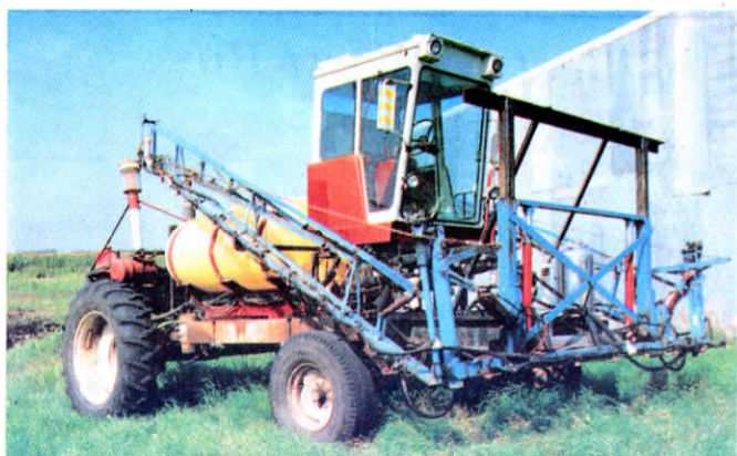
Klug removed both axles from 1972 IH 815 combine and mounted original front drive axle on back, then mounted front steering axle off old Allis-Chalmers tractor on front.
