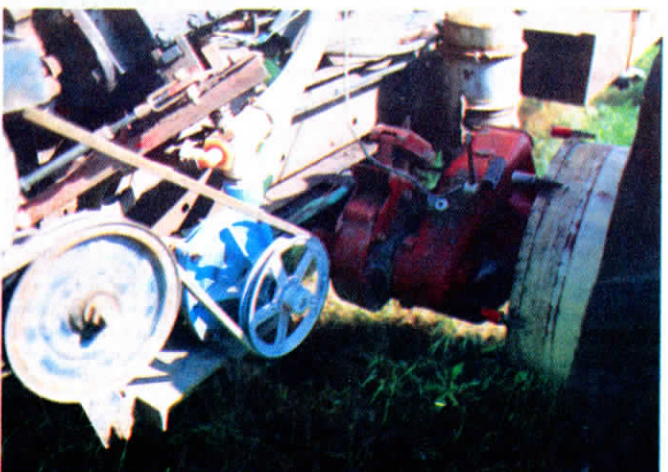
Klug widened combine's drive axle by moving wheel rims out as far as possible on axle housings. He then welded truck wheels onto the inside of each rim. Note magnets for Raven ground speed monitoring system mounted on inside edge of truck wheel.
