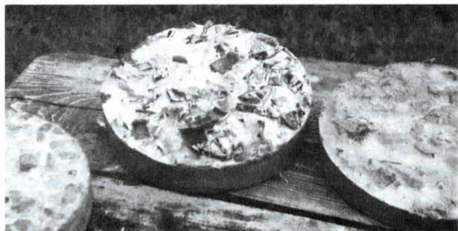
Sample slabs show "rubber rock" imbedded in concrete to create a cushiony surface that eliminates the need for rubber mats for livestock and also creates a non-slip surface. The rubber is mixed right into the concrete along with sand and water.
