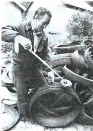
Geister checks treads with an inexpensive metal detector to separate steel-belted tires from bias ply tires.
