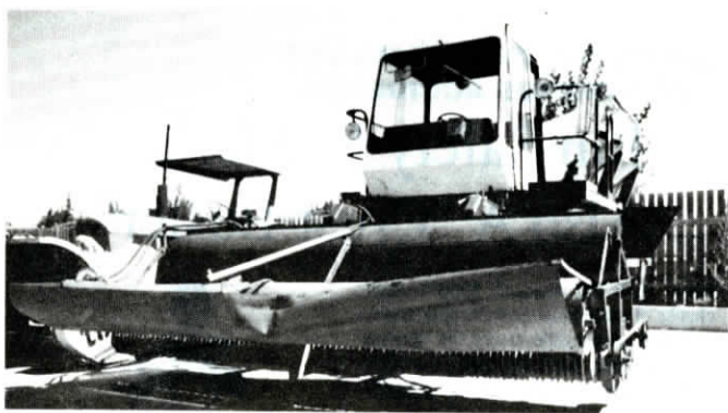
This prototype 12-ft. wide "stripper combine" is about the size and weight of a conventional grain head.
