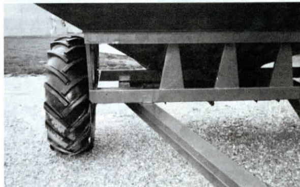
Frame and wagon mount on an axle made out of two Deere 55 combine front axles.
