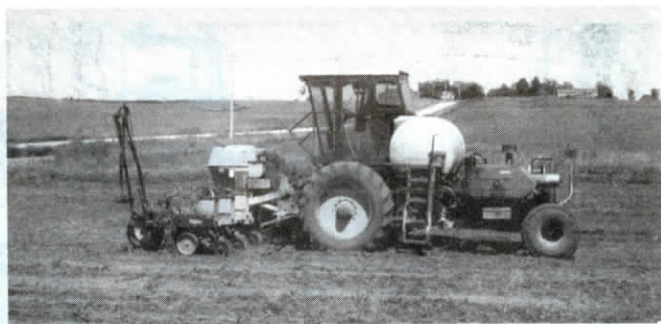
Augustine converted his 1979 Massey-Ferguson 760 combine into a self-propelled 8-row planter that also doubles as a 55-ft. sprayer with a spray boom.
