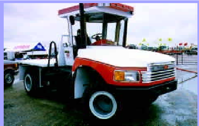
"Ranch Hand" has a 136-in. wheelbase and rides on 48 by 25.5 by 20 high flotation tires. It comes with leaf spring suspension and front and rear stabilizer bars.
