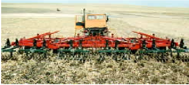
Kurkowski use a 125 hp. Unimog to pull this 28-ft. field finisher across corn stalks.
