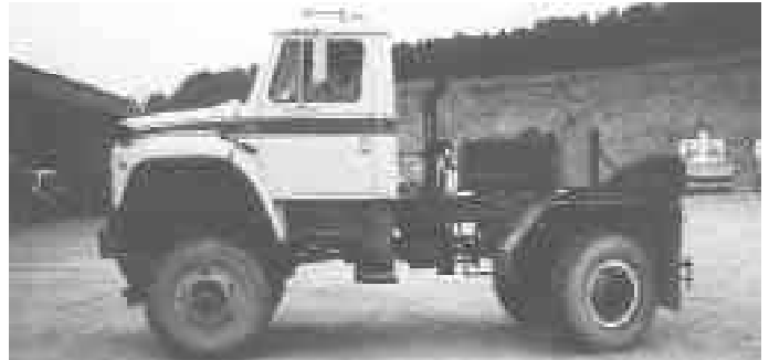
A pair of 2 1/2-ton steering axles from old Army trucks provide 4-wheel steering. 4-WD, 4-Wheel Steer “Utility Truck”
