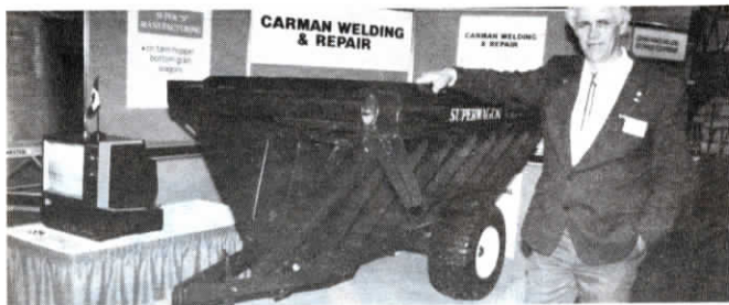
Scale model of "Superwagon" shows fold-down unloading auger fitted with feed-out spout for feeding into bunks.
