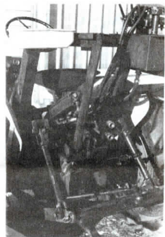
Long mounted a reservoir, 3-spool hydraulic controls, and pair of outlets above the rear axle just behind the seat.
