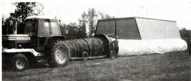
Offset bagger bags an entire row of bales at once, lifting each bale as it passes and setting it back down inside the long tubular bag.
