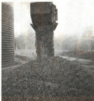
Sloped sides of unit and deflector plates let grain flow out of auger more gently.
