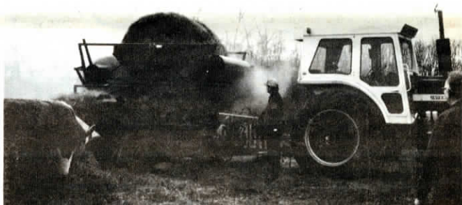
Eight large rollers rotate the bale while hay is stripped off for feeding.
