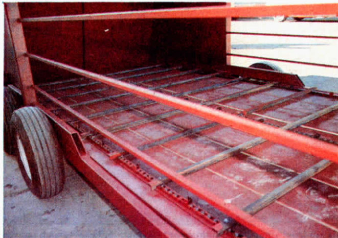
Stackbed apron is used both to form the stack, by moving loose hay to the rear, and to unload.
