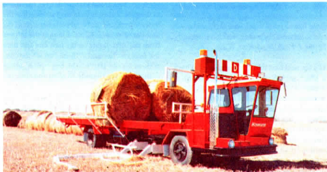
Big 12-bale rig was built on the frame of a garbage truck fitted with a combine cab.
