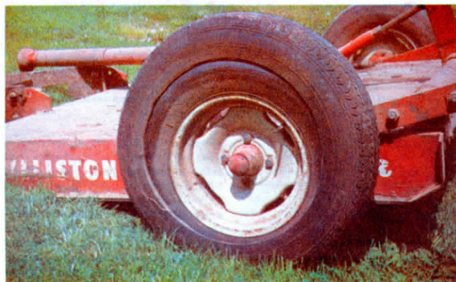
Cregger puts old tire casings over the tires on his mower to protect them.
