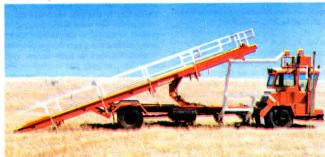
To unload, bed of truck is tipped up and four unloader chains pull bales off onto ground as truck drives ahead.
