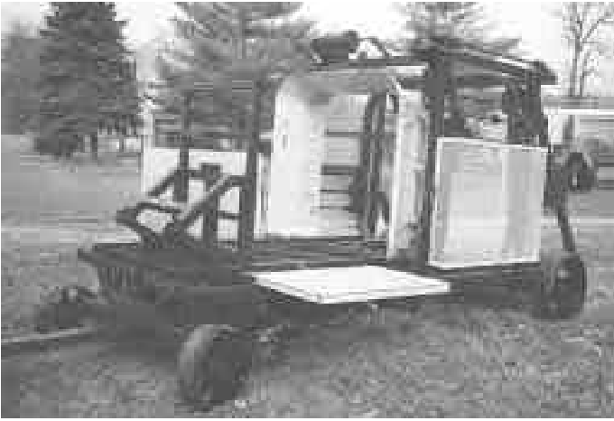
Powered by a 20 hp Kohler engine, "Master Wrap" adapts to different size bales by simply adjusting five bolts in squeeze chute.
