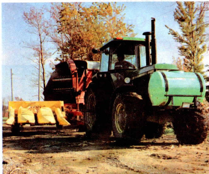
Enter widened New Holland 2-row snapper corn head to accommodate three 30-in. rows and mounted a used Deere corn silage cutting row unit in the middle.
