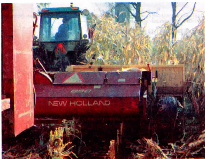
Combo harvester allows both corn silage and high moisture corn to be put up in same silo. Feed is three fourths kernels and one fourth silage by weight.
