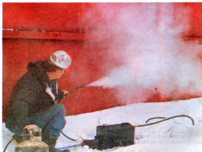
"Arctic Blaster" uses propane torch to create super-heated low-pressure dry steam.
