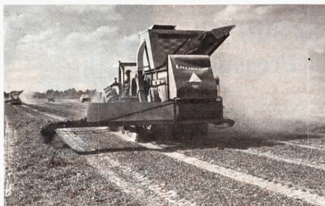
Cross conveyor is tested on a peanut combine. Normally, peanut hay would be raked into windrows, causing damage and loss of leaves.
