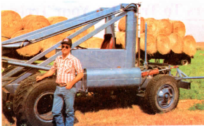
Rodocker used the axles and suspension system from a White semi and a 455 cu. in. engine from a junked Oldsmobile Toronado to build his machine.
