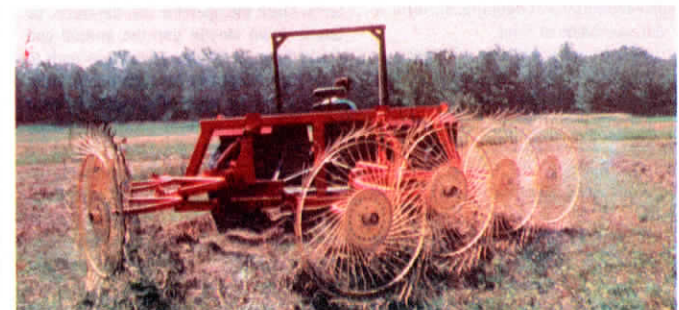
Crown used heavy 4 by 4-in. sq. tubing to build his 18-ft. wide two-rake hitch.
