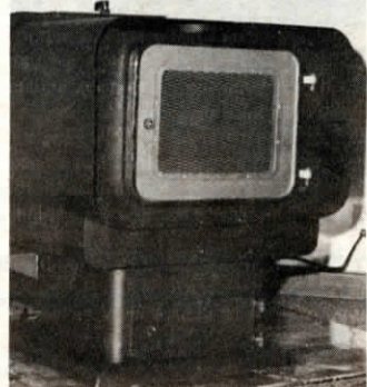
A feed auger carries corn to a pre-burning chamber that gasifies the fuel. Smoke and gases generated burn in a secondary combustion chamber that exhausts the heat through a heat exchanger that blows out into the room.
