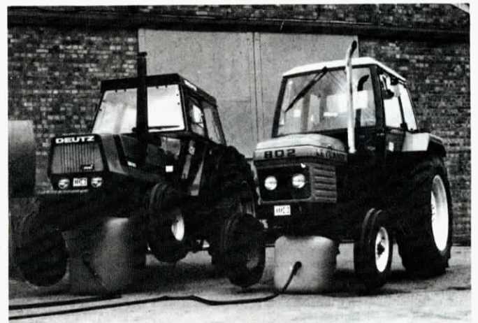
Fitted to auto exhaust pipes, jacks easily lift tractor front ends.
