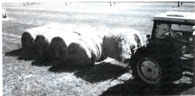
"Sled" carries eight 4 by 5-ft. bales and a ninth bale is carried on a 3-pt. bale fork.
