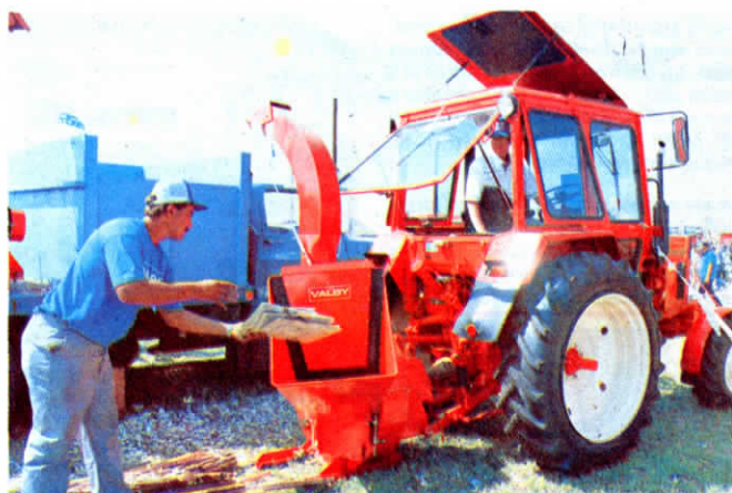
Some farmers and custom operators use brush chippers to shred newspaper. You can run a tube directly from the discharge chute to a baler to bale up the shredded paper.
