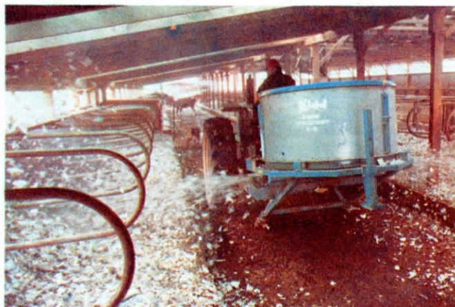
Lee Shaffer fills his Kidd bale chopper with 300 to 400 lbs. of newspaper that's blown into stalls. Smaller single-bale choppers can also be used to shred newsprint.
