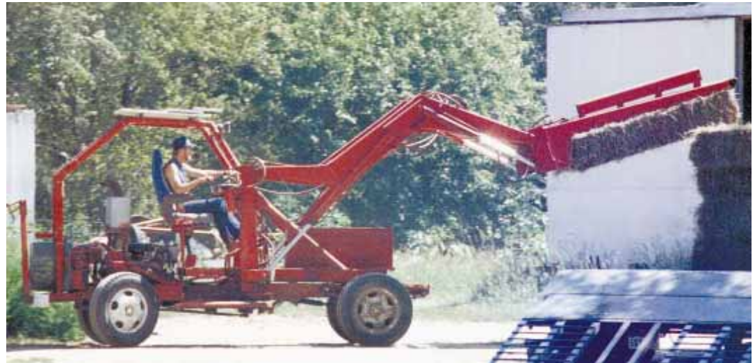
Regier says the bale loader can reach out farther and higher than a tractor-mounted bale grabber. “I can lift the bale fork 20 ft. high and stack bales 11 high - right to the top of our shed,” he says. “It also works great for loading bales on my gooseneck trailer.”
