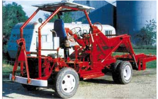
Self-propelled bale loader was built out of an old 1 1/2-ton Ford truck chassis, a front-end loader, and a Farmhand 8-bale grabber.
