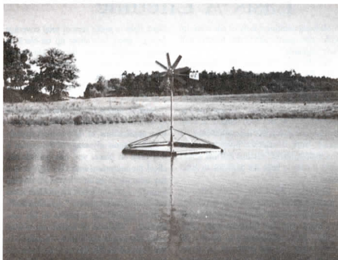
Underwater propeller creates swirling vortex that keeps water circulating in pond.
