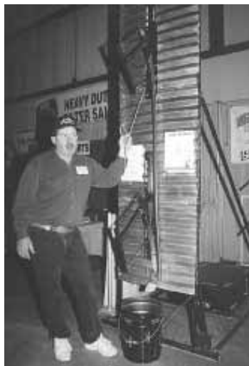
Preston's 4-ft. long probe enters the bin at an upward angle for quick, safe sampling.
