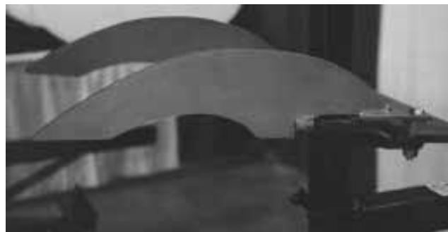
Mounted 1 ft. apart on the header, bolt-on “Grain Lifter Guards” consist of half-moon-shaped pieces designed to run 1/2 to 1 in. below the cutterbar.
