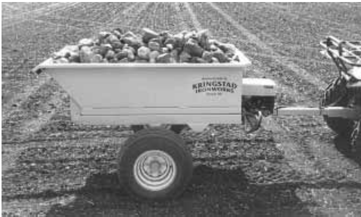
Cart has a 1,500 lb. load capacity but adds only 150 lbs. to back of ATV thanks to its balanced design. It dumps at the press of a button.
