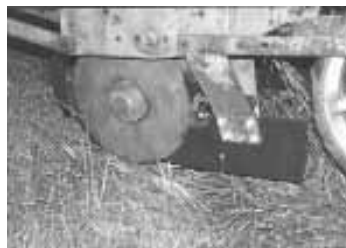
Conventional planter shoe was redesigned so that it’s only 1/2 in. wide. Discs open a groove just wide enough to accommodate the shoe.
