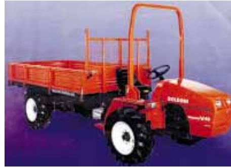
Box on Goldoni "Transcar" dumps to right, left, rear.
