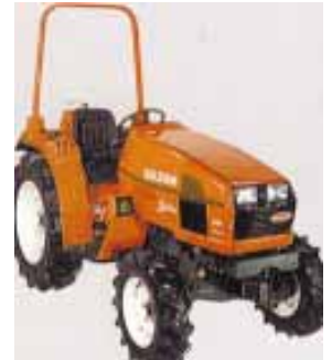
Mini tractor haulers are powered by 21, 30 or 37 hp diesel engines.
