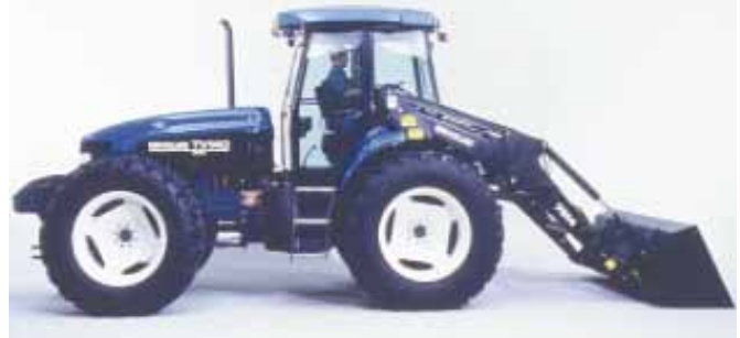
The cab on this New Holland TV 140 features new "Turnabout" console that turns with seat so tractor controls are identical no matter which direction you're traveling.
