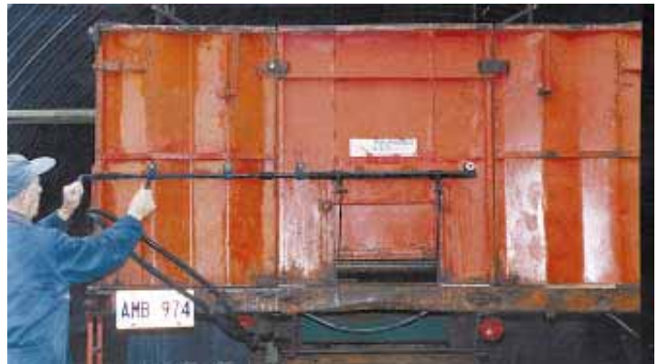
Steel shaft runs horizontally across back of box and has a lever welded onto one end. To lock the door in any desired position, Routledge mounted a locking lever on the shaft.
