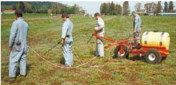
The 3-wheel hydrostatic unit is powered by a 10 hp gas engine. It allows several operators to spot spray weeds at the same time working from one unit.
