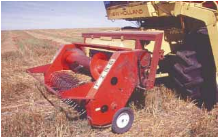
Mounting a Gehl forage harvester pickup head on his New Holland TR-70 combine lets Johnson harvest windrowed oats much earlier than he could by direct-cutting them.
