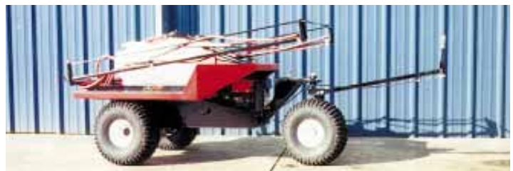
Tanks mount on a dump bed. With the tanks removed you can use the rig as a powered wheelbarrow. Note: Photo shows latest new production model.
