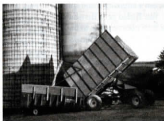
Photo shows wagon with plywood sides in place.
